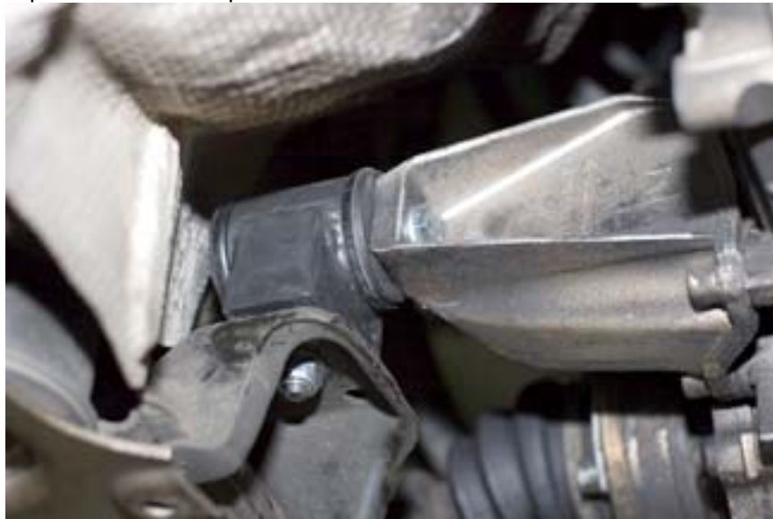
PHOTO 4 – Stern mount installed
